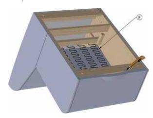
**E:** Using a knife (a box cutter will work much better for this), slice the foam away wherever it is glued to the frame.
