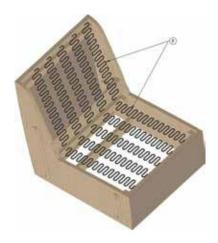
**F:** Once the foam is removed, the next step is to remove the sinuous springs mounted to the seat and back.
